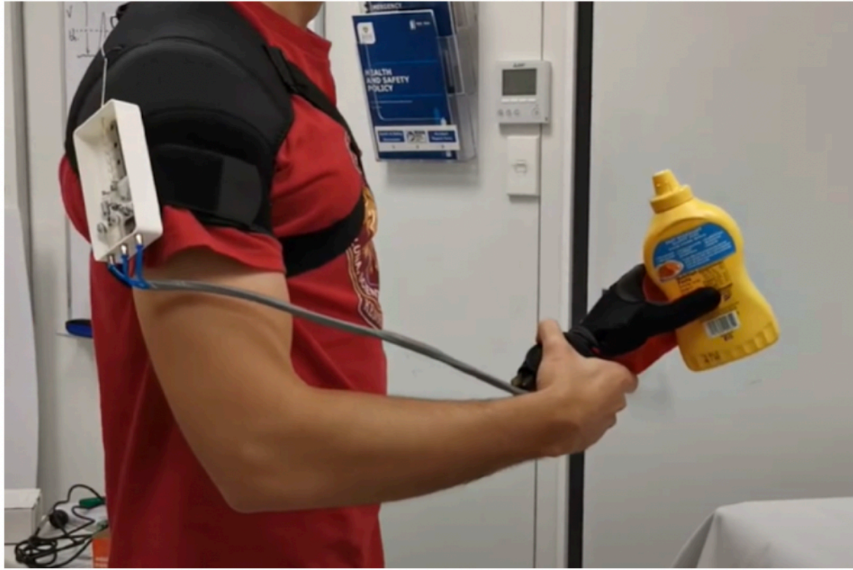
Figure 2. The OpenBionics body-powered partial hand prosthesis (left subfigure) and wearable exoskeleton glove (right subfigure).
